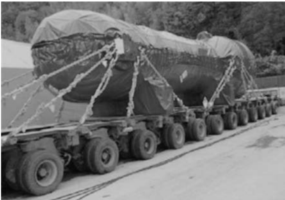
Fig. 10 Chooz-A SGs transport to ANDRA VLLW Repository
