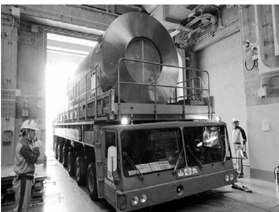
Fig. 5 Spent fuel transfer from Unit 1 to Unit 3
